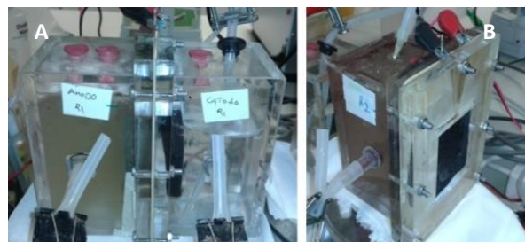
Figure 1 - A: MFC H-form separated by a Nafion membrane; B: MFC with an anode chamber and cathode in direct contact with air.
